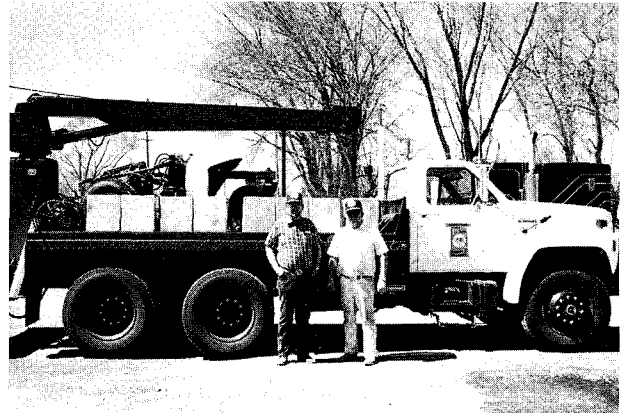
The weight cart on the truck, built by an employee, helps on livestock auction scales.
